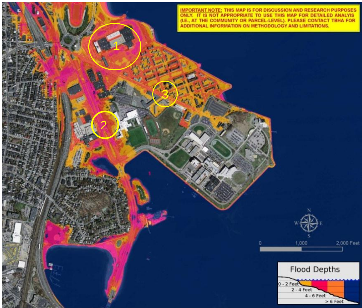
Figure 18. Projected surface flooding at UMass Boston due to future 2.5 ft of sea level rise plus 5 ft storm surge (MHHW+7.5/12.3 ft NAVD). Vulnerable areas include Bayside Expo (1), Morrissey Blvd (2) and Mt. Vernon St (3).
