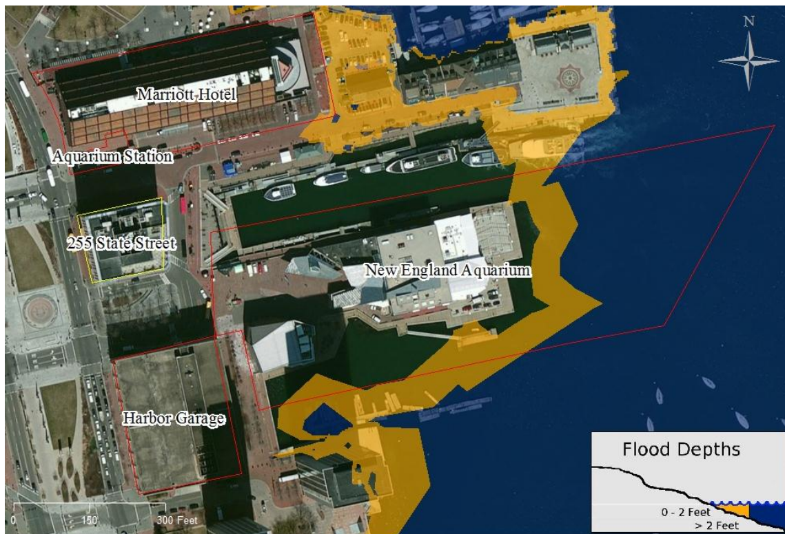
Figure 13. Estimated area of tidal flooding by mid- to late-century (Kirshen et al.; MHHW+2.5/7.3 ft NAVD)
